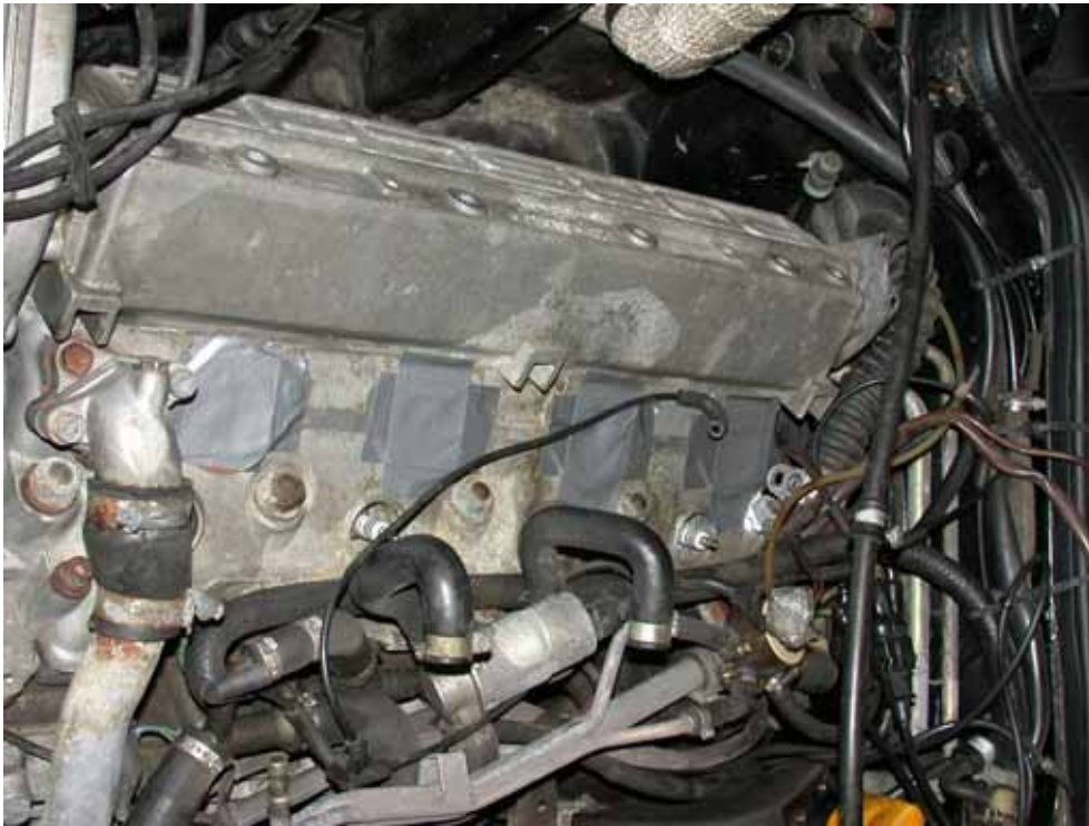
Image 8 - Cover the intake holes to prevent contamination of intake chamber
