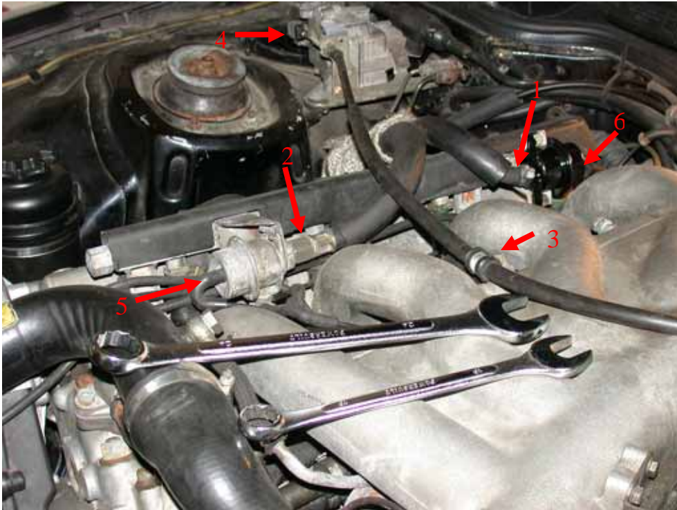
Image 2 - Fuel rail and fuel lines. 1. Fuel return line. 2. Fuel line nut. 3. Cruise control line hold-down bolt. 4. Cruise control servo unit. 5. Vacuum line to fuel damper. 6. Vacuum line to fuel pressure regulator.
