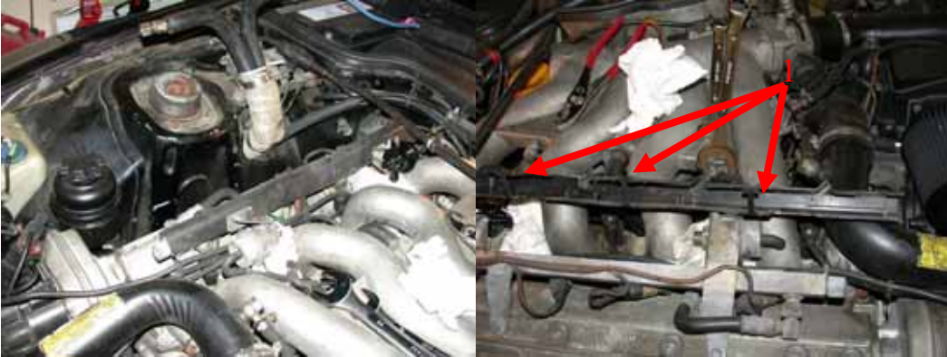
Image 3 - Fuel lines removed and attached out of the way and fuel rail cover
