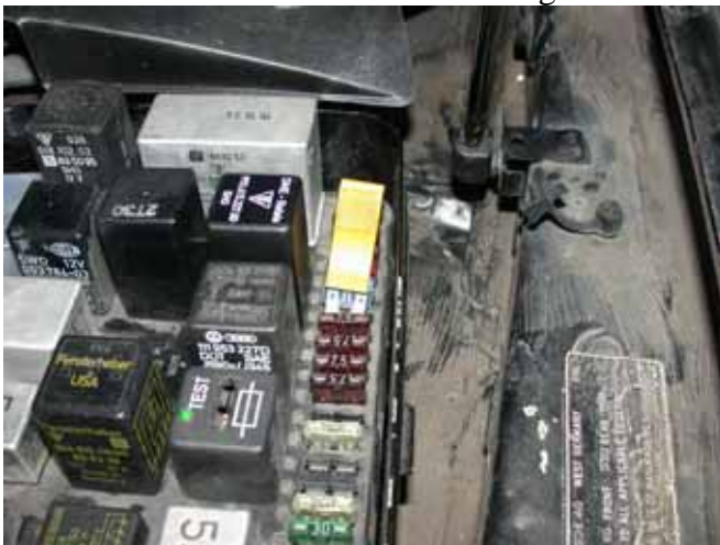
Image 1 - Removing the fuel pump fuse at #34
