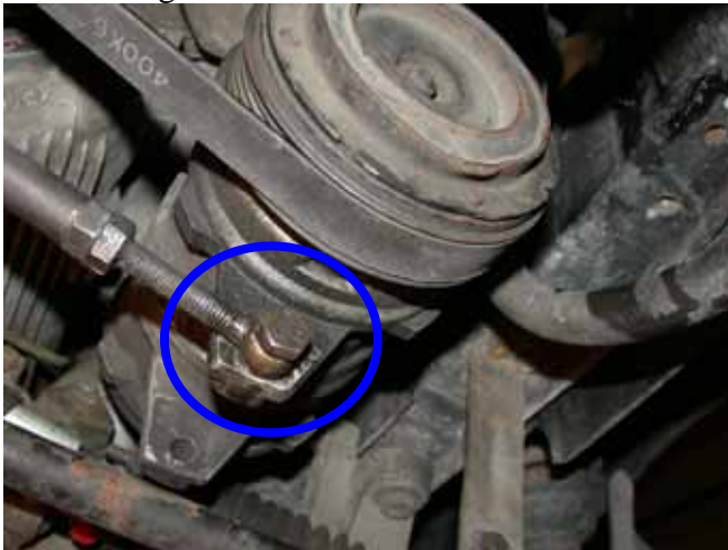
Image 13 - A/C compressor turnbuckle bolt
