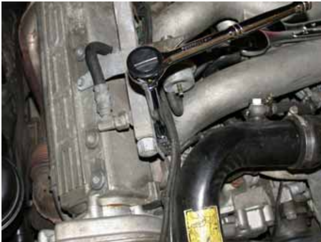
Image 5 - Unbolting the forward fuel rail to intake manifold bolt.
