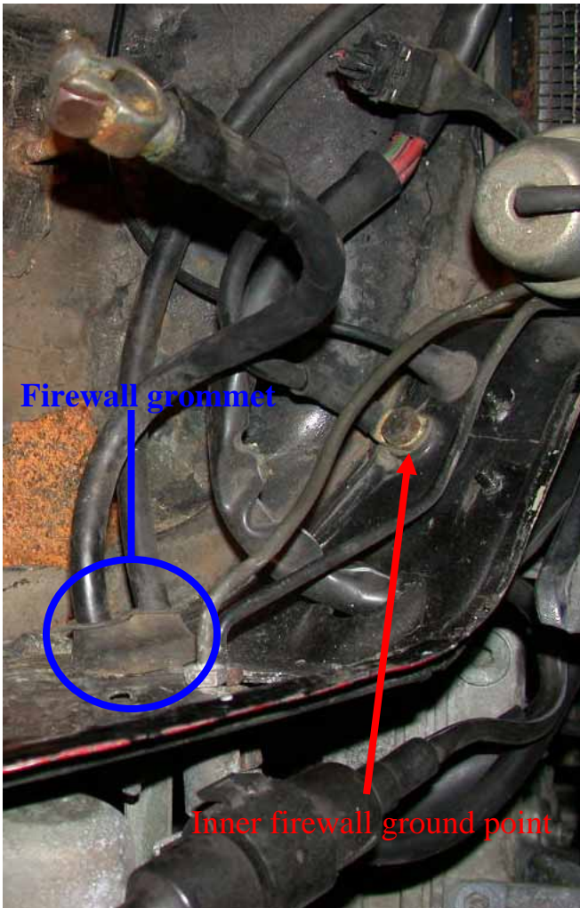
Image 11 - Inner firewall ground point and grommet
