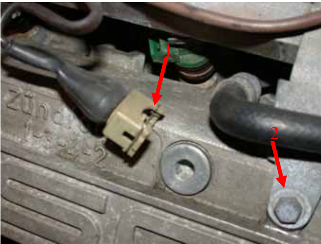
Image 4 - Unclipped connector for fuel injector. Notice the metal retaining wire around the connector (#1 in Image).
