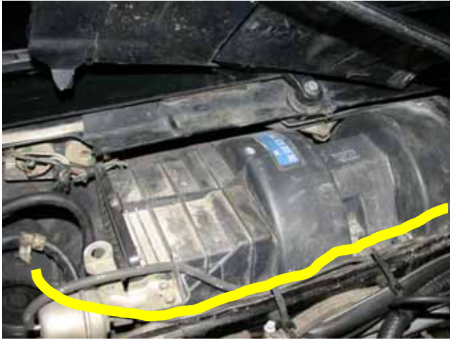
Image 21 - Plastic debris cover lifted up to expose the blower motor area.
